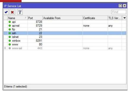
The Wiki uses a singular command of /ip service disable telnet,ftp,www,api,api-ssl to efficiently disable these self-descriptive services in one pass. Understanding the functions of these services will better enable you, as the Administrator of the network, to determine if you will utilize these services.
