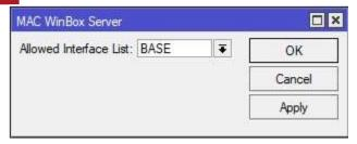
Modify the value of the **Allowed Interface List** by **left clicking** the list box arrow at the end of the field. **Left click** on the value of **none**. This default interface sets the associated service to not use any of the internal or external connections available to the device. **Left click** the **OK** button to commit the change.
