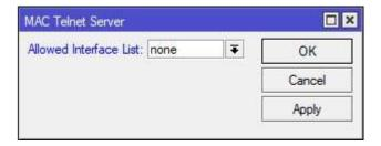
As shown in the image above, modify the value of the **Allowed Interface List** by **left clicking** the list box arrow at the end of the field. **Left click** on the value of **none**. This default interface sets the associated service to not use any of the internal or external connections available to the device. **Left click** the **OK** button to commit the change.
