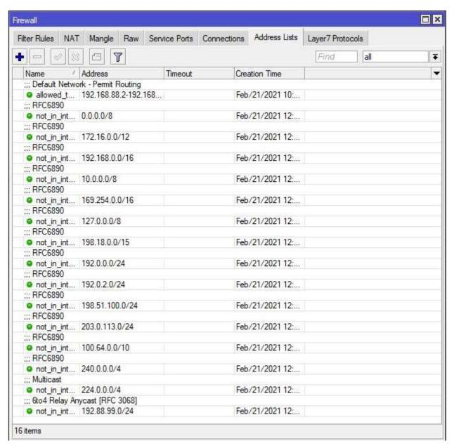
If the command block is altered to only contain a comment for the first *not\_in\_internet* range, the *Multicast* range, and the *6to4 Relay Anycast [RFC 3068]* range, then the resulting presentation in the **Address Lists** tab will appear as shown below.
