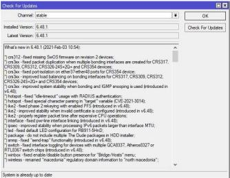
To apply a newer release (when available) within the stable channel, left click the **Download&Install** button in order to obtain and apply the noted updates. Upon completion of installation, the device will reboot. A disconnect will occur within WinBox after the update has been completed. Reconnect to the device once it is online and reappears in the **Neighbors** tab.
