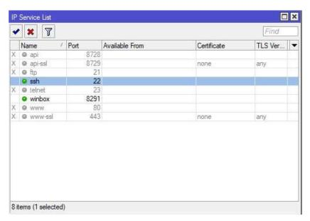
**NOTE**: While this screenshot shows the ssh service running on the default port, the recommendation in the <u>SSH</u> procedure to change the port number will result in the port value being different than what is displayed in this example.
