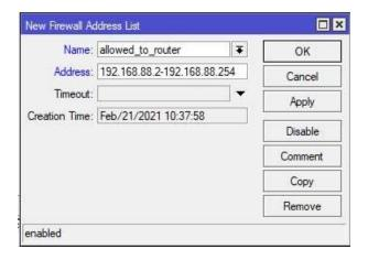
**Left click** the **OK** button to establish the Address List. The comment that was entered will appear above the entry in the Address Lists. If you have defined additional networks and DHCP servers to support ranges beyond the default configuration, the subsequent additions to the **allowed\_to\_router** list can be made by selecting the established name in the drop-down list and entering the additional network(s) that have been established.
