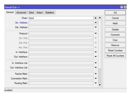
To the right of the text fields in the **General** tab is a scroll bar. Scrolling further down toward the bottom will provide visibility for the **Connection State** line. In this line, the check boxes for **established**, **related**, and **untracked** are selected. The following line in the Wiki code block is slightly more secure than the default configuration as it excludes untracked connections.
